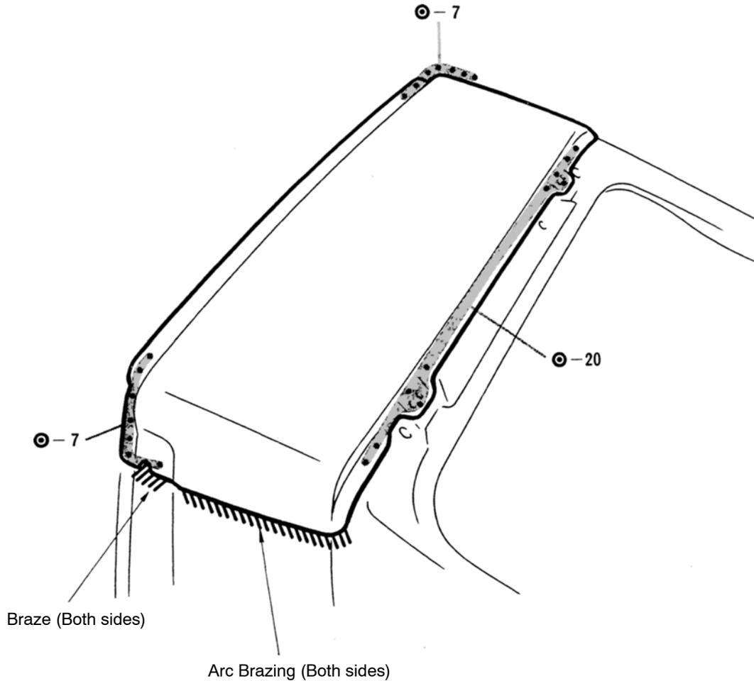
1. Heat the braze area of the quarter panel and scrape off the brazing with a wire brush.
