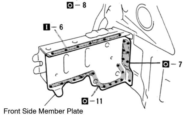
1. Before temporarily installing the new part, weld the front side member reinforcement to front side member.
