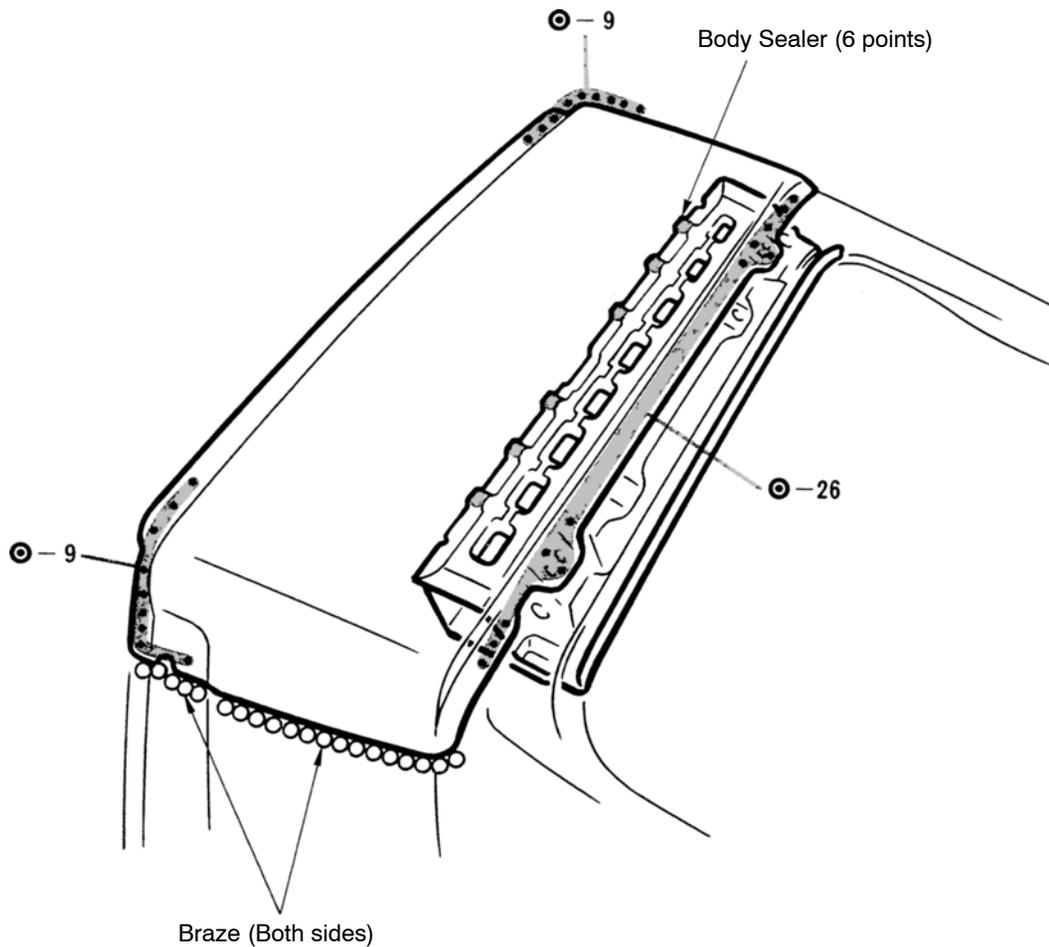
1. Before temporarily installing the new part, apply body sealer to the back door opening frame.
