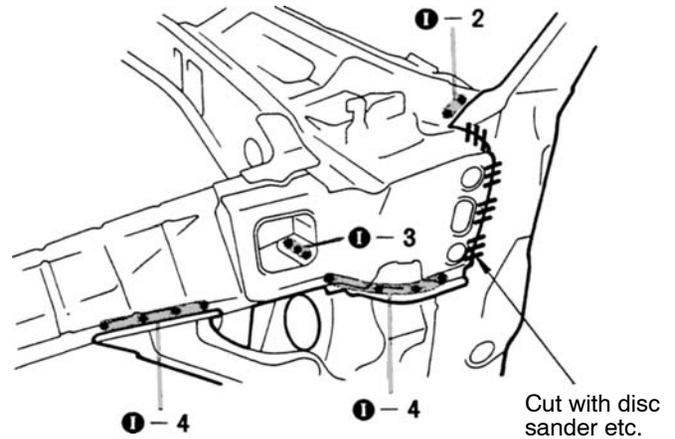
1. Replace the front body pillar together with front body pillar reinforcement lower inner.
