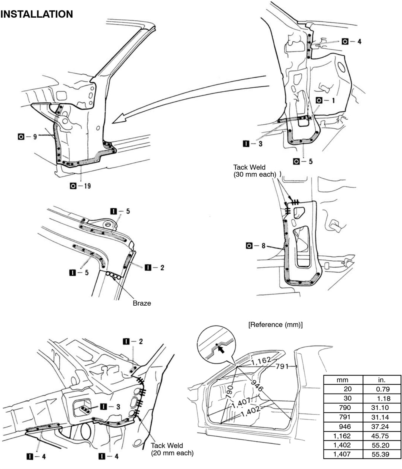
1. Temporarily install the new part and check the fit of the removable roof, front door, front fender, hood and windshield glass.
