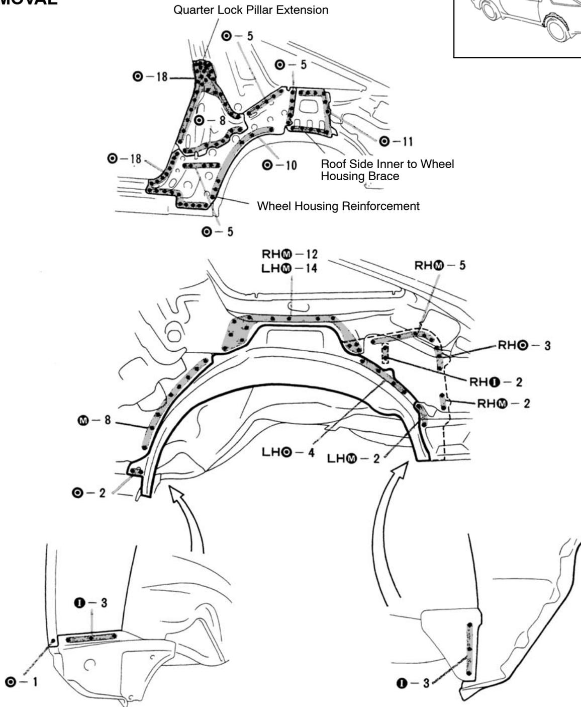
1. After removing the quarter lock pillar extension, wheel housing reinforcement and roof side inner to wheel housing brace, cut and join the quarter wheel housing outer panel.
