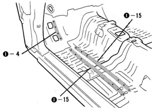
1. Replace the front floor under reinforcement together with the front side member reinforcement.
