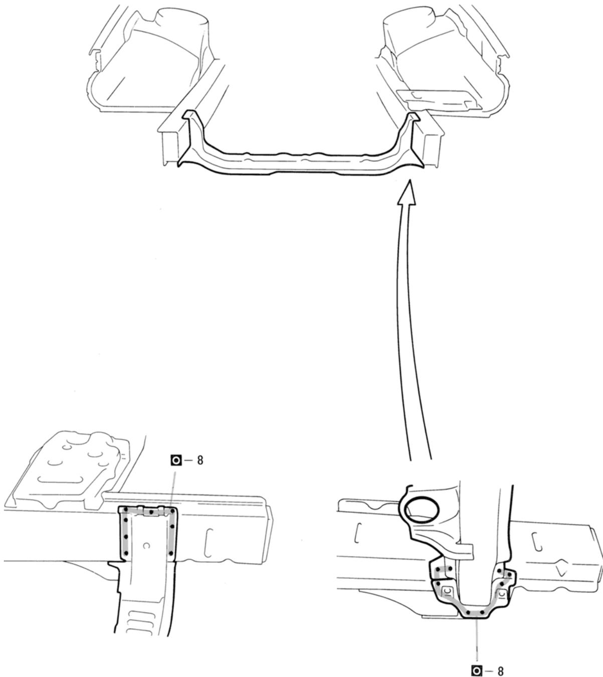
1. Temporarily installing the new part and measure each part in accordance with the body dimension diagram.
