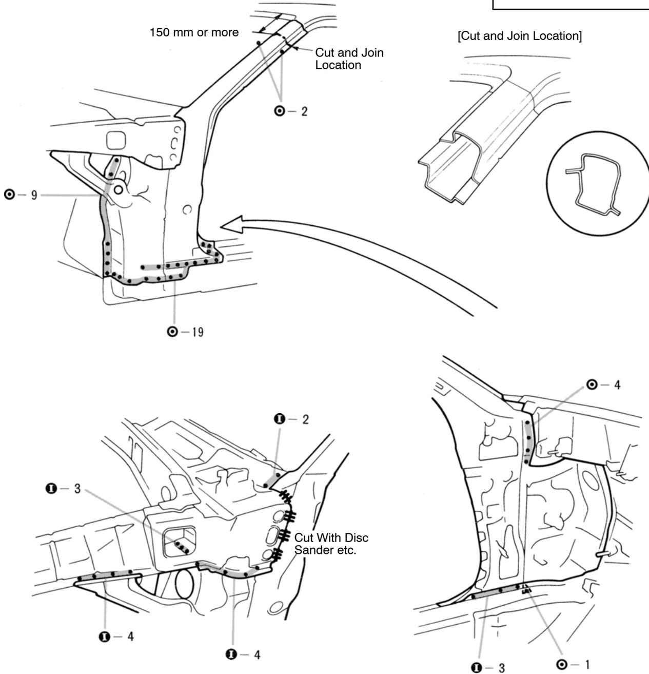
1. Cut and join the front body pillar at the location shown above.
