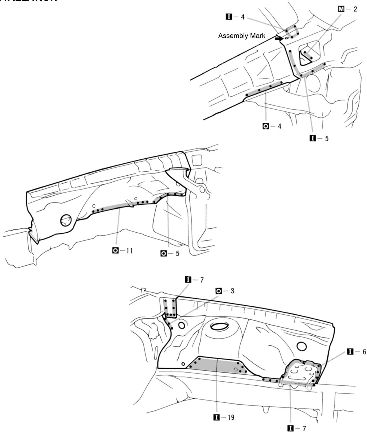
1. Determine the installation position of the new part by the assembly mark.
