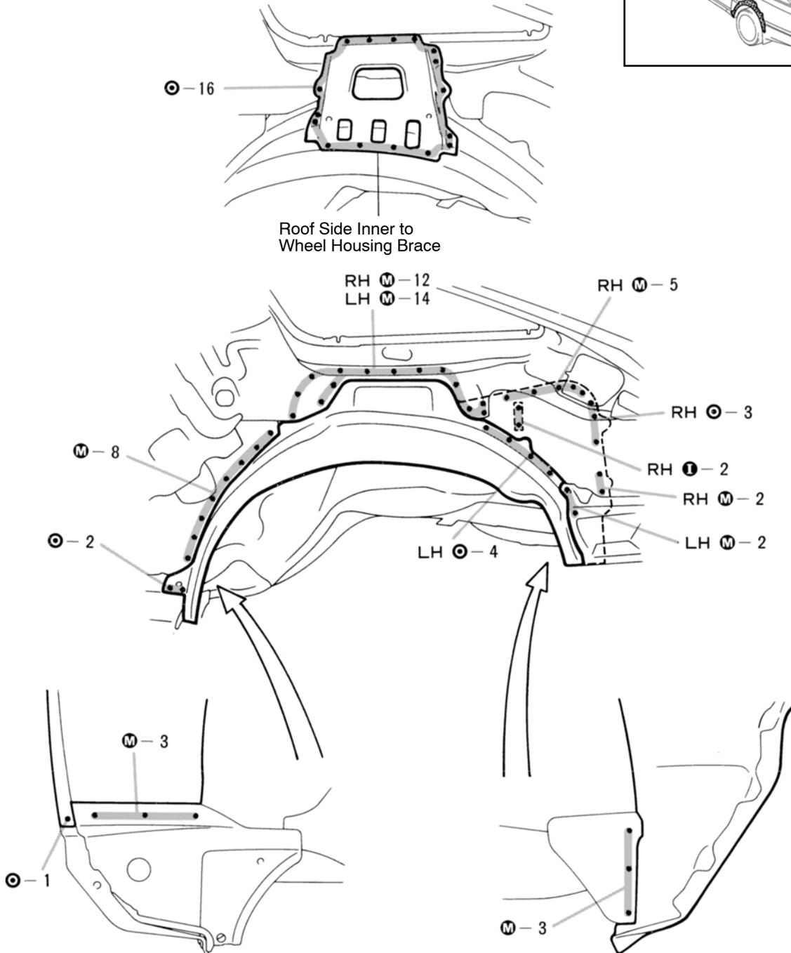
1. Before removing the quarter wheel housing outer panel, remove the roof side inner to wheel housing brace.
