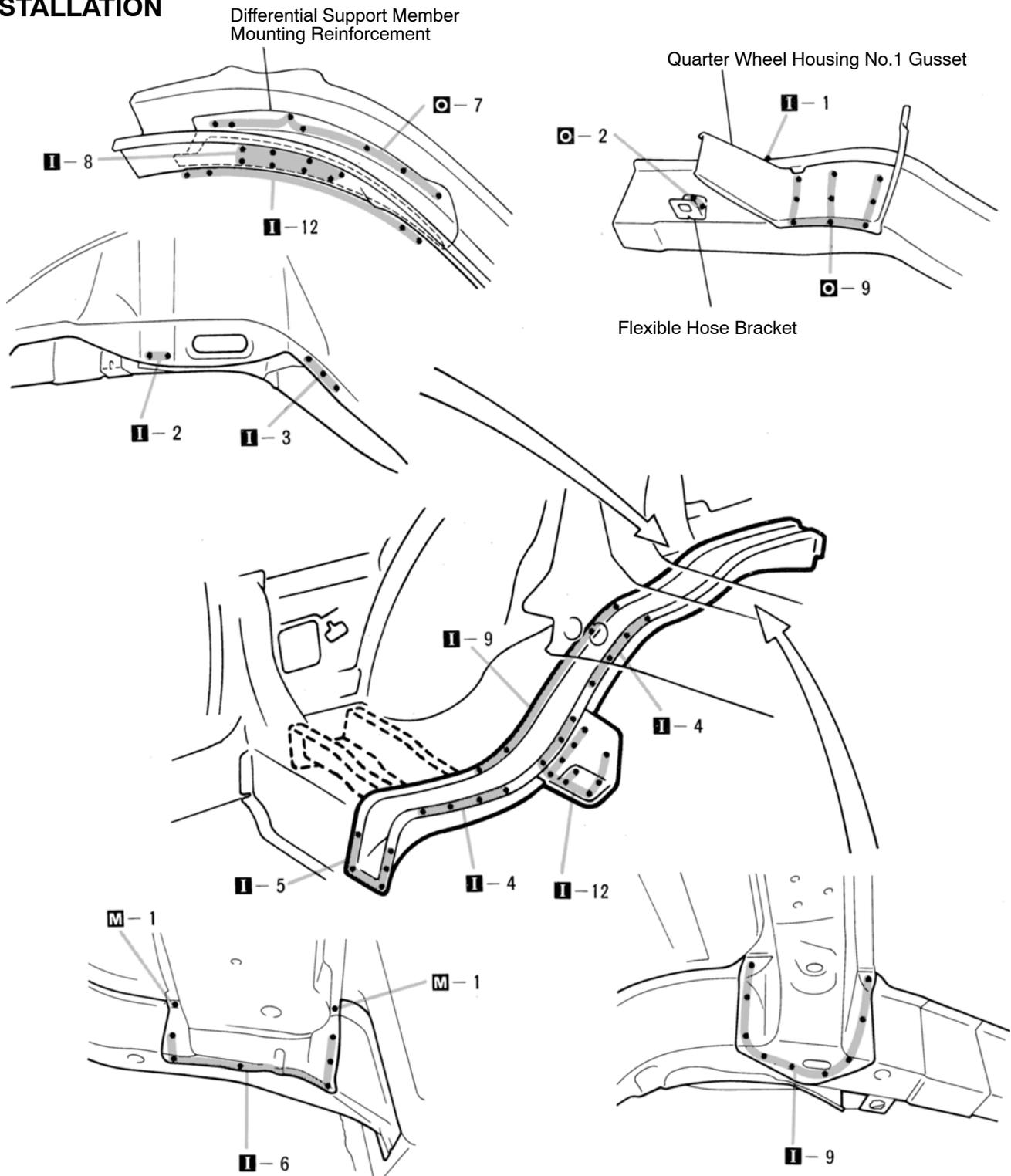
1. Temporarily install the new part and measure each part in accordance with the body dimension diagram.
