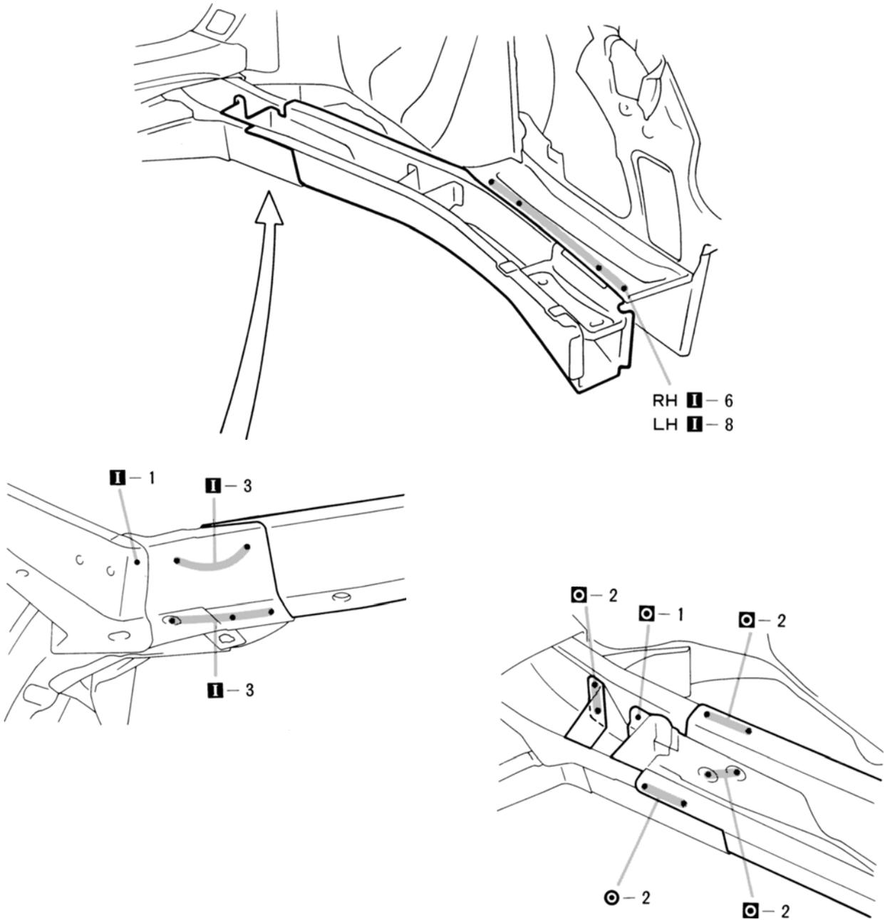
1. Temporarily install the new part and measure each part in accordance with the body dimension diagram.
