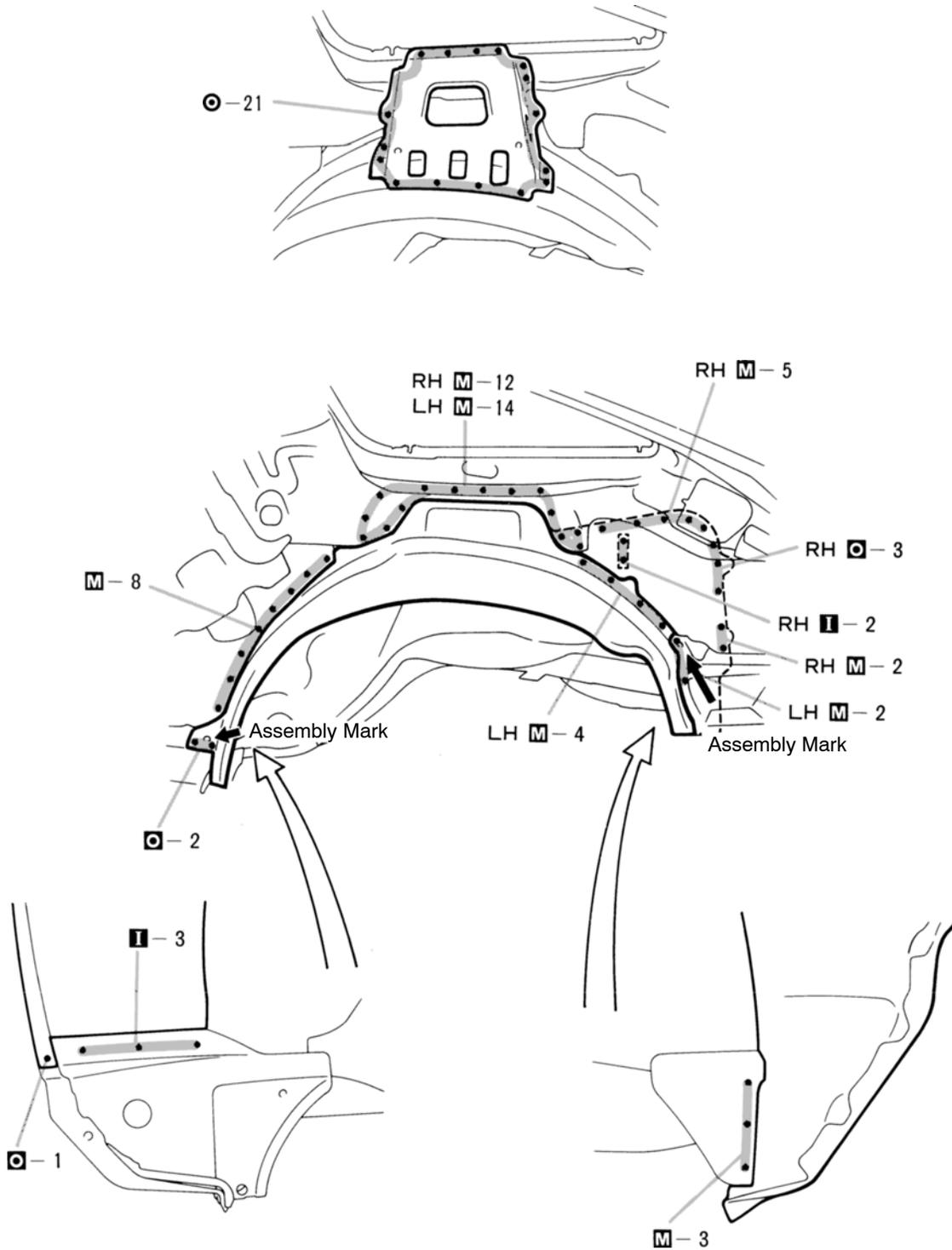
1. Determine the position of the new part by the assembly marks of the inner and outer panels.
