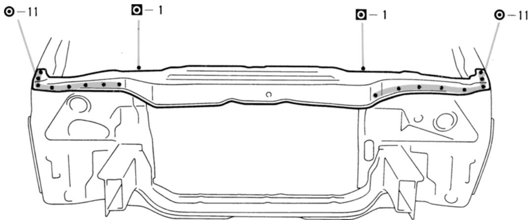
1. Temporarily install the new part and measure each part in accordance with the body dimension diagram.
