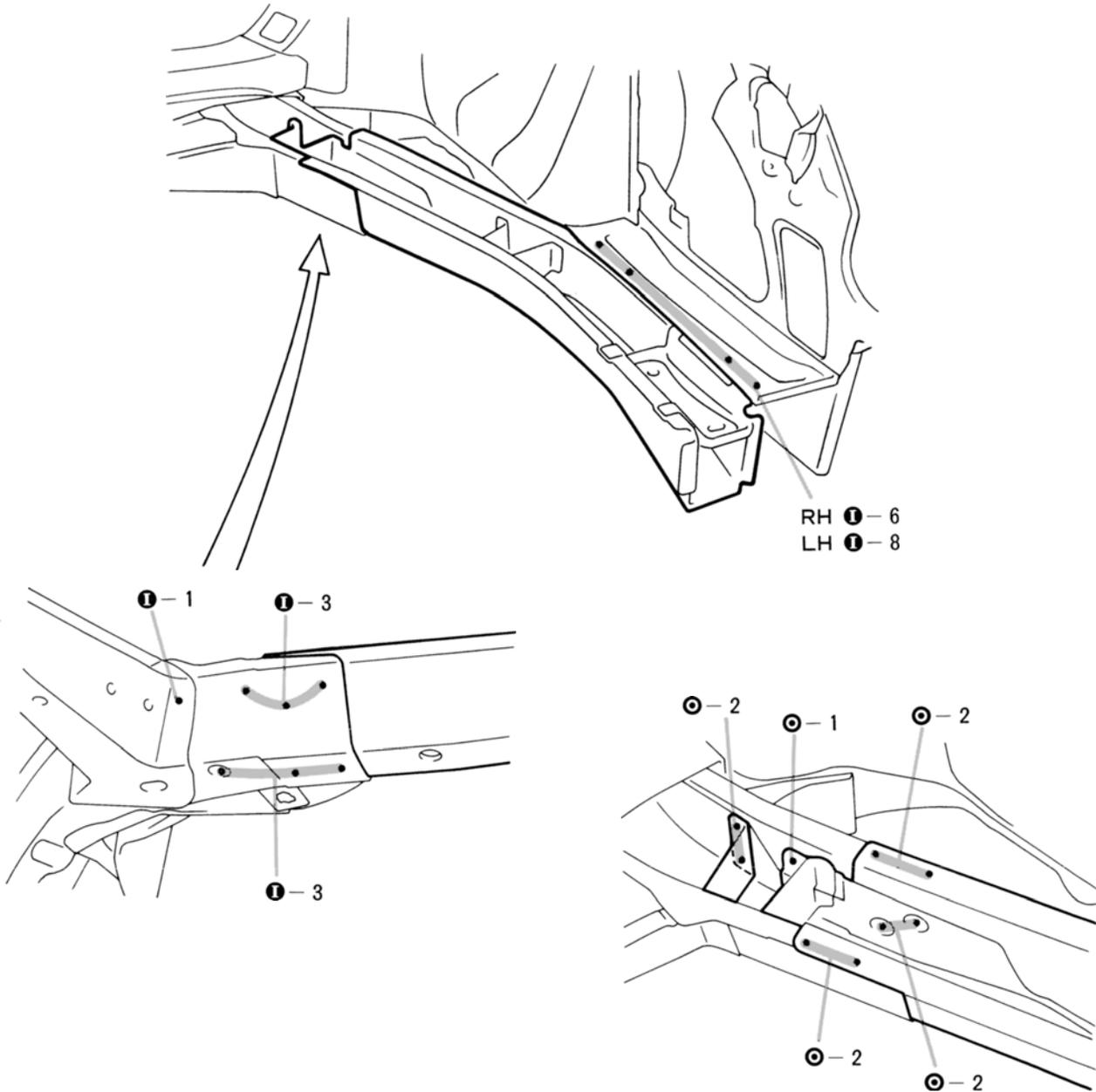
1. Before removing the rear floor side member, remove the rear floor pan.
