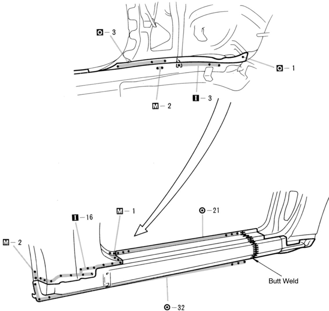
1. Temporarily install the new panel and check the fit for the front door and front fender.
