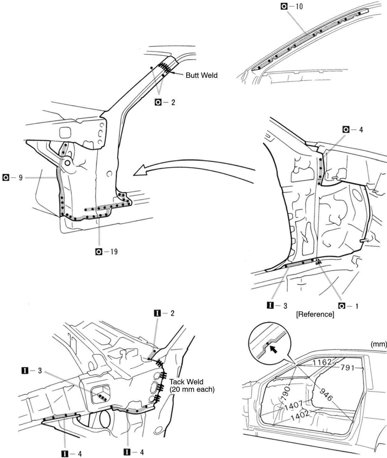
1. Temporarily install the new part and check the fit of the front door, front fender, hood and windshield glass.
