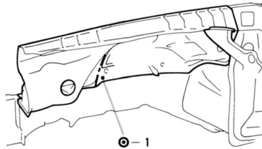
1. After removing the spot welds, rough cut the front fender apron shown above.
