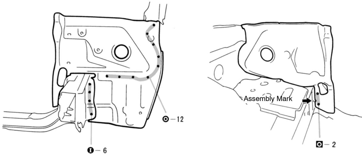
1. Temporarily install the new part with the assembly mark and measure each part in accordance with the body dimension diagram.
