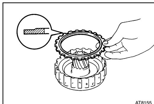
(b) Install the flange, the flat end facing downward.
