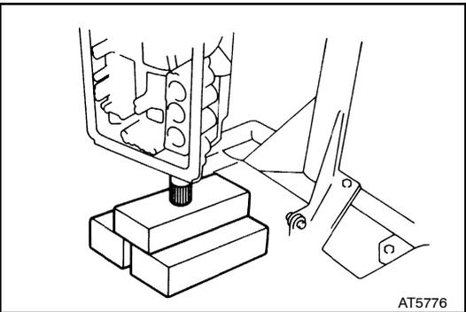
(e) With wooden blocks or equivalent under the output shaft, stand the transmission on the output shaft.
