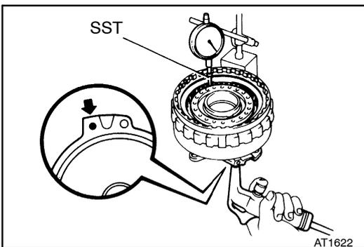
**4. CHECK PISTON STROKE OF TRANSFER DIRECT CLUTCH**
