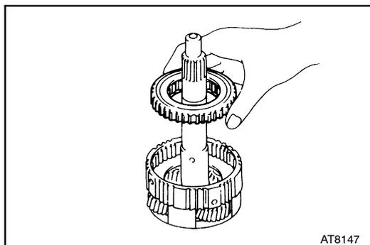
**9. REMOVE OVERDRIVE ONE-WAY CLUTCH WITH OUTER RACE**
