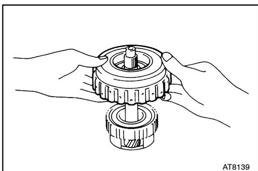
**9. INSTALL OVERDRIVE DIRECT CLUTCH ASSEMBLY**
