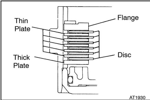
**3. INSTALL PLATES, DISCS AND FLANGE**
