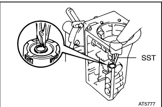
(f) Using SST, remove the snap ring.
