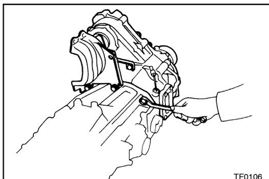
**9. REMOVE PROPELLER SHAFT UPPER DUST COVER AND TRANSFER FROM TRANSMISSION**
