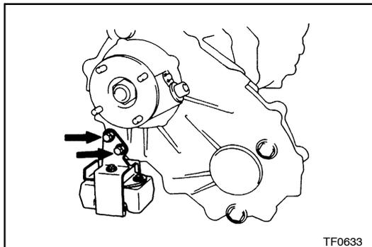
**8. REMOVE DYNAMIC DAMPER**
