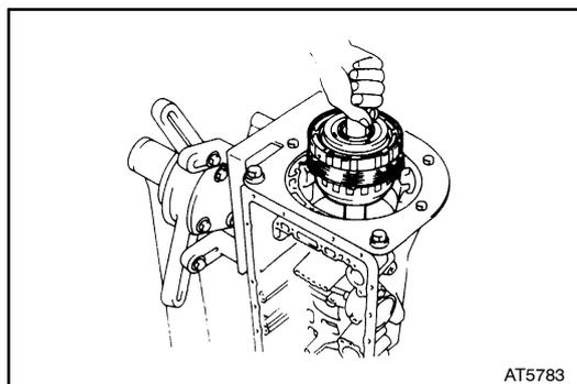
(d) Remove the assembled thrust bearing and race from the case.
