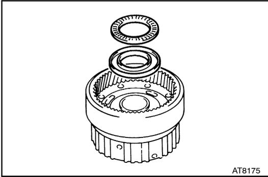
(c) Remove the bearing and race.
