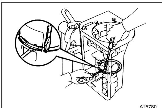
**36. REMOVE FLANGE, PLATES AND DISCS OF SECOND BRAKE**
