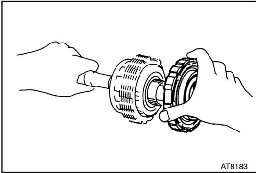
(e) Remove the second brake drum assembly.
