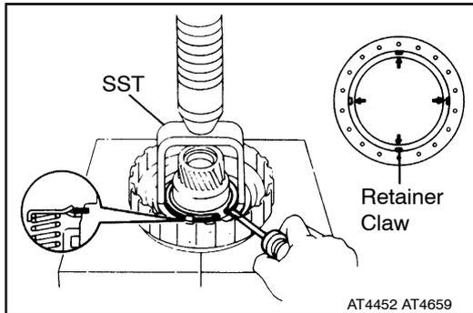
(b) Place SST on the spring retainer, and compress the return spring with a shop press.
