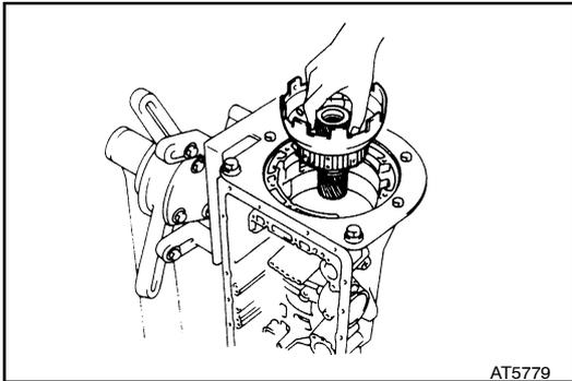
**34. REMOVE PLANETARY SUN GEAR WITH NO. 1 ONE-WAY CLUTCH**
