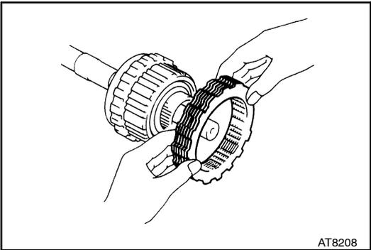
(f) Remove the cushion plate, flange, plates and discs of the first and reverse brake.
