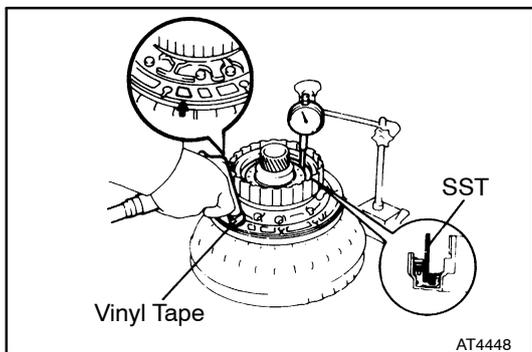
**8. CHECK PISTON STROKE OF OVERDRIVE DIRECT CLUTCH**
