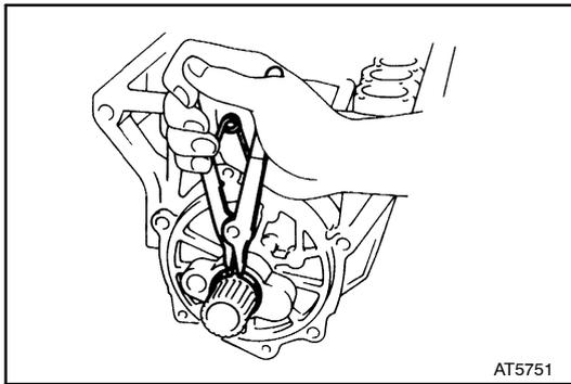
**11. REMOVE SPEED SENSOR ROTOR AND KEY**
