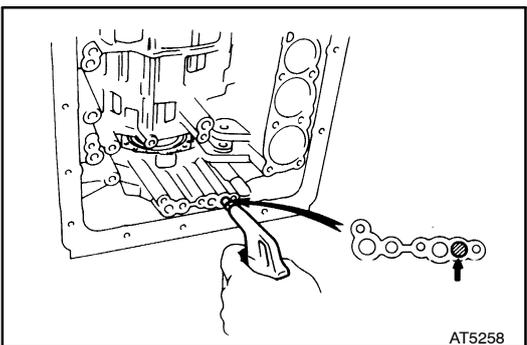
**42. CHECK PISTON STROKE OF FIRST AND REVERSE BRAKE**
