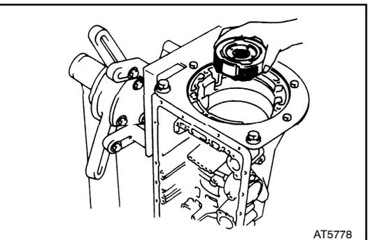
(g) Remove the front planetary gear from the case.
