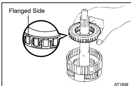
(b) Install the overdrive one-way clutch with the outer race to the overdrive planetary gear.
