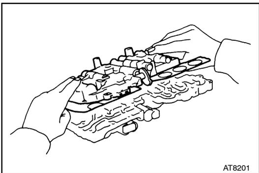
4. **PLACE UPPER VALVE BODY WITH PLATE AND GASKETS ON TOP OF LOWER VALVE BODY**
