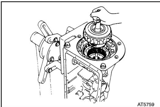
**25. REMOVE OVERDRIVE PLANETARY GEAR UNIT WITH OVERDRIVE DIRECT CLUTCH AND ONE-WAY CLUTCH**
