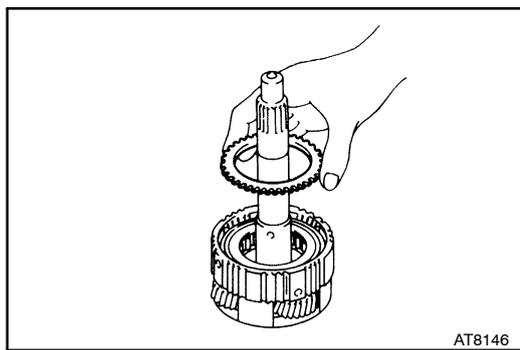
(b) Remove the retaining plate.
