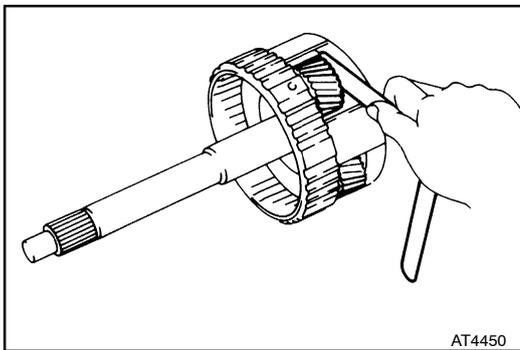
**5. MEASURE PLANETARY PINION GEAR THRUST CLEARANCE**
