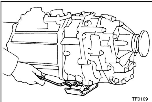
**7. REMOVE ENGINE REAR MOUNTING**
