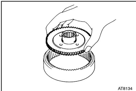
(b) Remove the ring gear flange.
